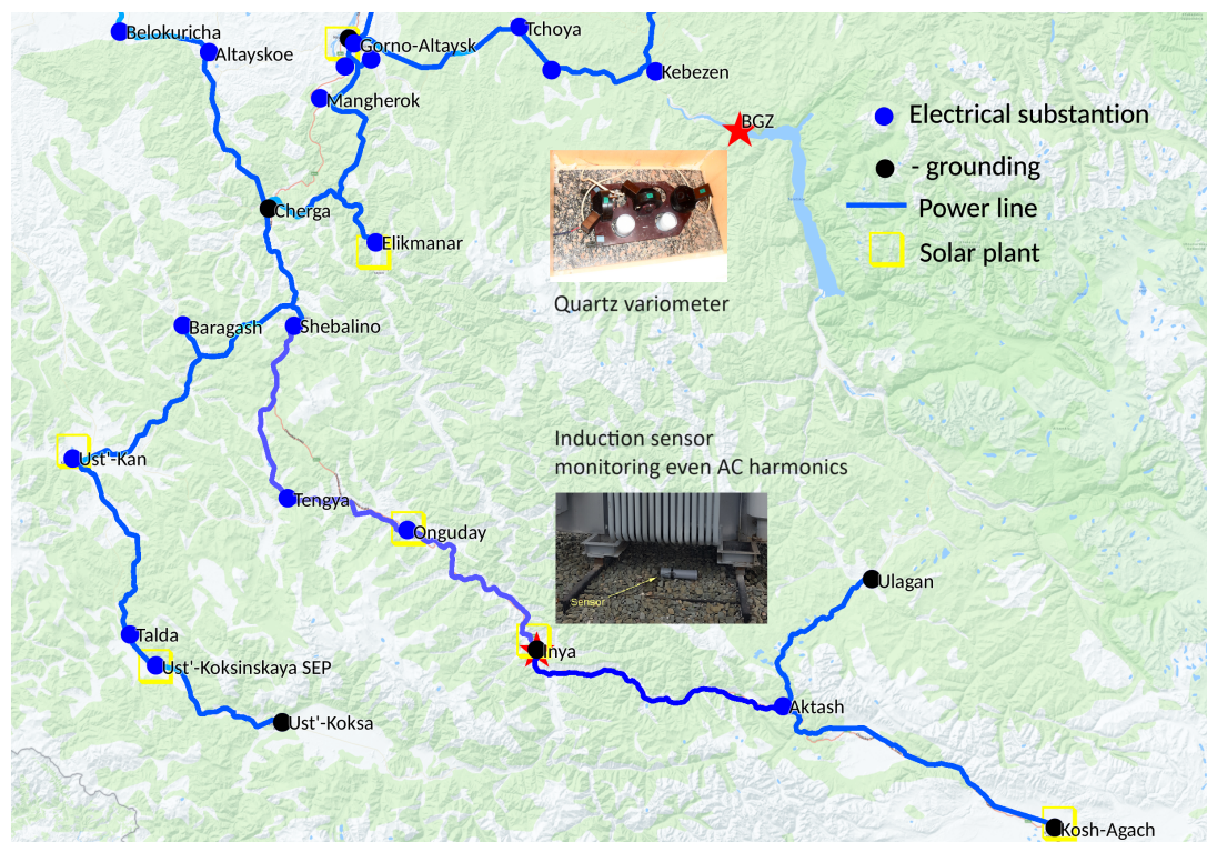
Fig. 1. Scheme of the location of the monitoring points of geomagnetic variations (BGZ) and the even AC harmonics amplitude in the power grid of the Altai Republic (Inya). There are shown the power lines 110 kV, power substations, solar plants.
