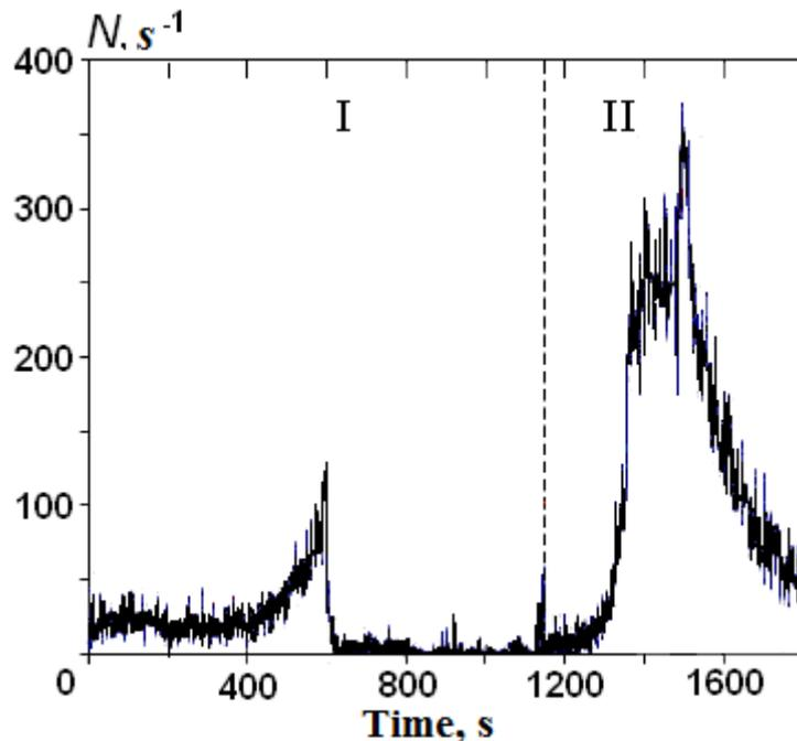
Fig. 4. Change of AE activity in time during monoaxial coal deformation in the second cycle (II) after a triaxial axisymmetric compression in the first cycle (I) [12]
