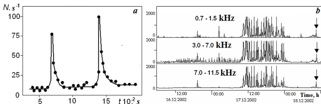
Fig. 3. *a*) Fracture formation rate in a diabase when a sample is constantly influenced by monoaxial compressive stress [7]. *b*) Geoacoustic signals registered before the earthquake on 18.12.2002 ( $K = 12.1$ ) in Kamchatka (IKIR). The event time is indicated by an arrow [11]
