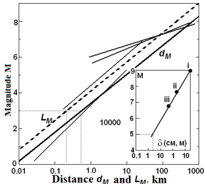
Fig. 1. Earthquake magnitude  $M$ , geoblock size  $d_M$ , fracture length  $L_M$  [1]. Thin lines are the data on fracture length of different authors. On the insert: dependence of  $M - \delta$ . Dots show earthquake parameters in Sumatra (i), Altai (ii) and California (iii).
