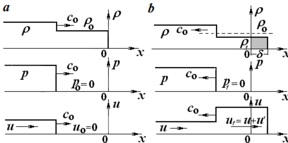
Fig. 2. Profiles of density, pressure and velocity during a weak shock wave emergence at a free surface a) before the emergence  $t < 0$ ; b) after the emergence  $t > 0$  [4]. The section marked by gray shows that media loosening occurred after a SW passage, and a layer with the thickness  $\delta$  and the density  $\rho_1 < \rho_0$  was formed
